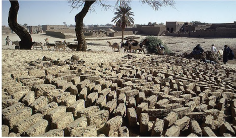
Figure 6. Locally produced sun-dried brick by Timbuktu people.
