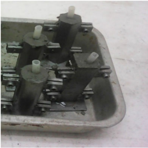
Figure 1. Piles cast with pipes at top.
