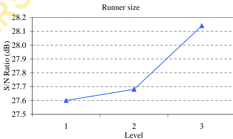
Figure 2c. Main effects plot for runner size S/N ratio values on impact energy
