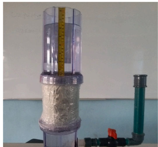
Fig. 4. Scheme of hydraulic conductivity test.
